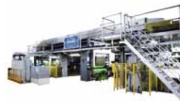
Unsupported alufoil coating machine
